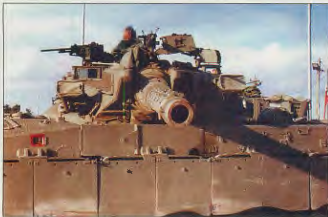
Protective skirts protect running gear; ever-ready flexible MAG protects troops manning site.
